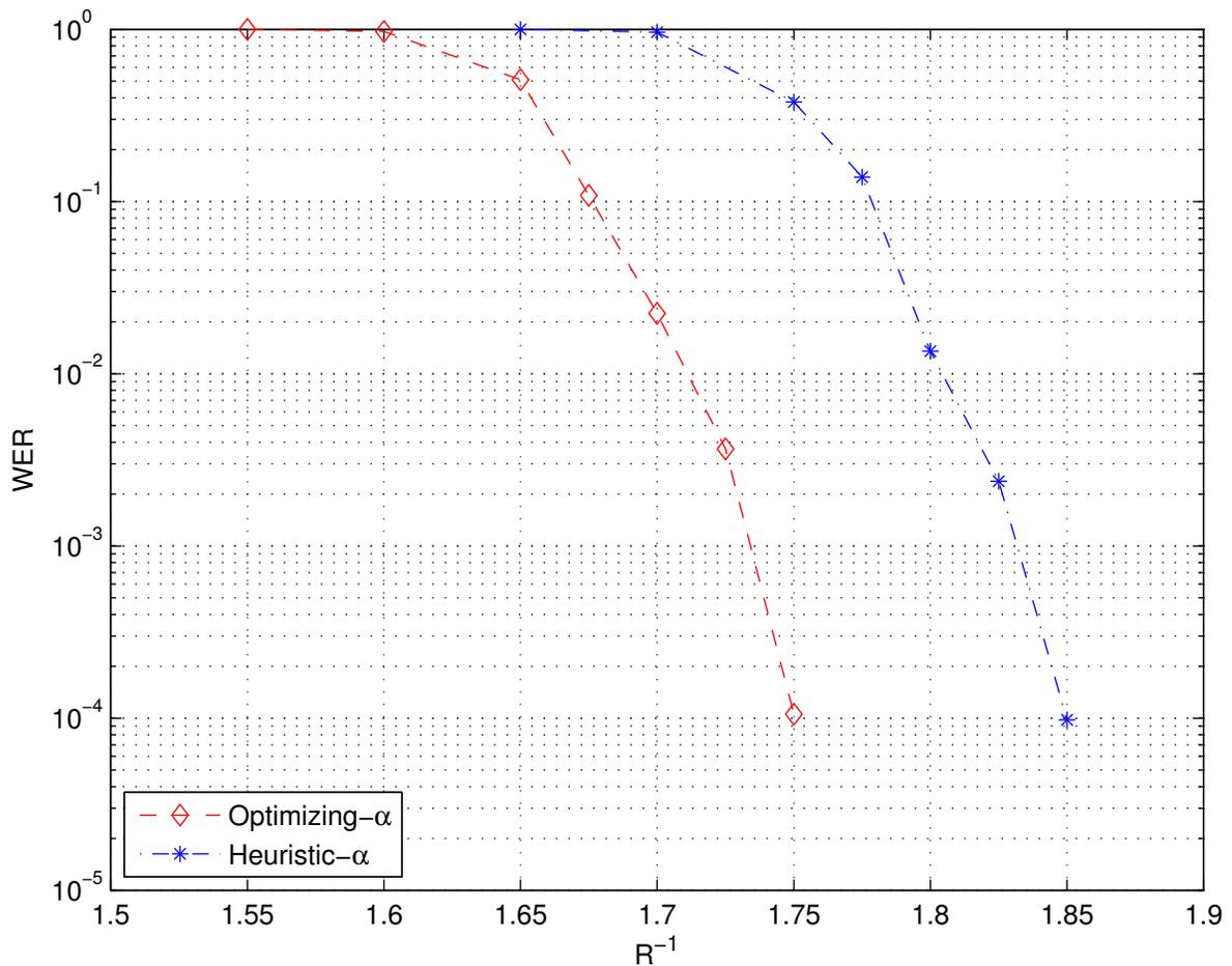
Fig. 6. Word error rate of the Raptor code as a function of  $1/R$  for the two approaches over channel with SNR=2.5 dB.
