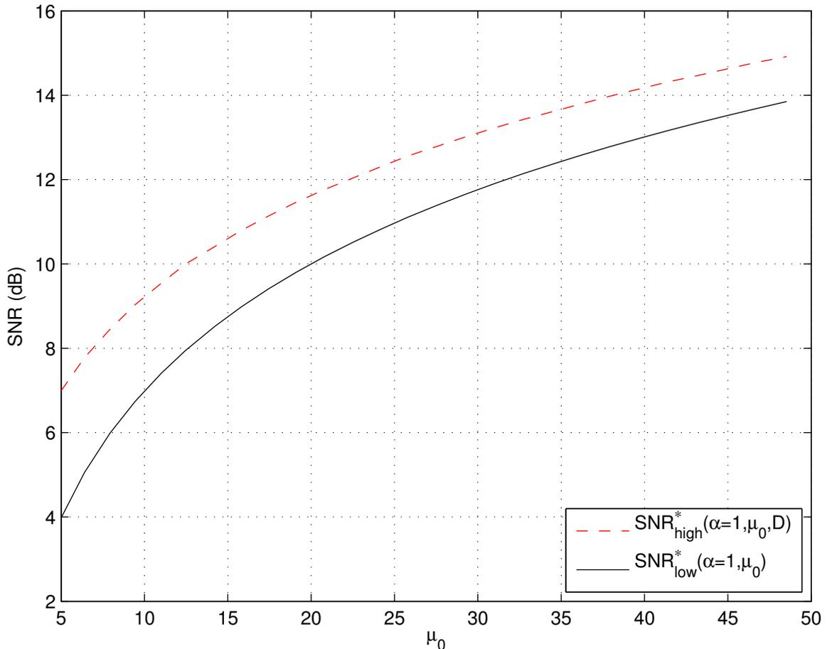
Fig. 2. Bounds  $\text{SNR}_{\text{high}}^*(\alpha, \mu_0, D)$  and  $\text{SNR}_{\text{low}}^*(\alpha, \mu_0)$  as functions of  $\mu_0$  for  $\alpha = 1$ .
