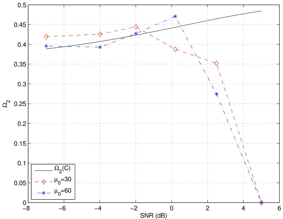
Fig. 4. Determined  $\Omega_2$  with different  $\mu_0$  at various values of channel SNR.
