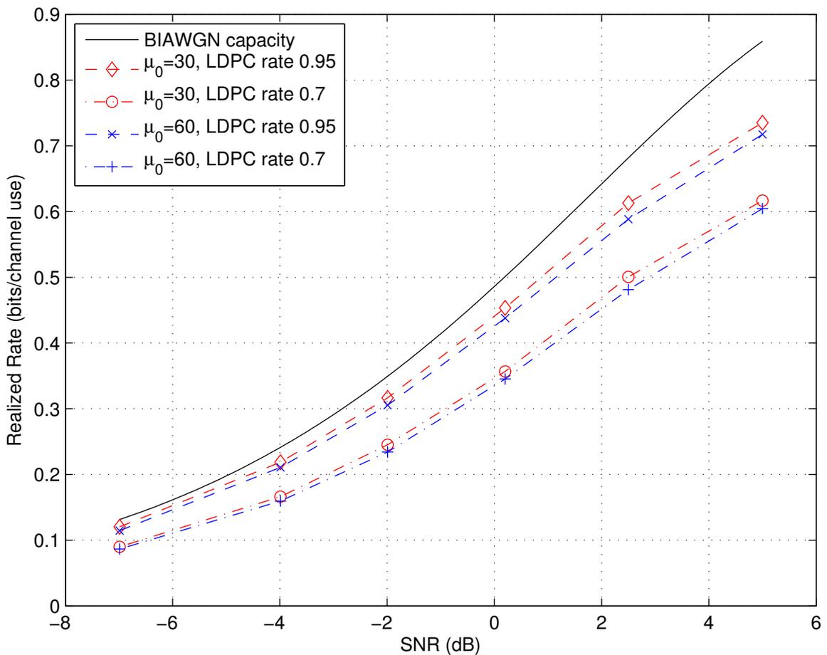
Fig. 3. Realized rates of Raptor codes constructed using different parameters.
