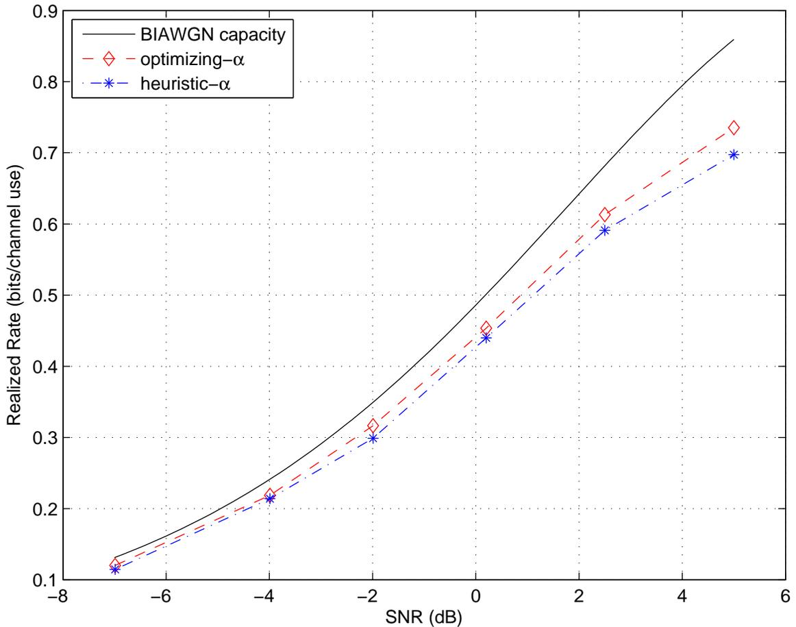
Fig. 5. Realized rates of Raptor codes constructed respectively using heuristic- $\alpha$  and optimizing- $\alpha$  approaches.
