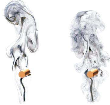
Fig. 8. Three-dimensional flow patterns of a vertical vortex jet around a static cylinder of unit radius. Kernel radius is  $\epsilon = 1$  and  $c_{slip} = 0.0$  (left) and  $c_{slip} = 1.0$  (right).
