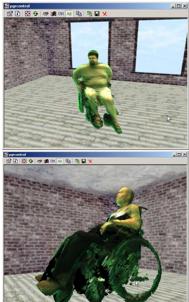
Figure 4: Remote view screen capture from TightVNC client (top: optimized view, bottom: non-optimized view).
