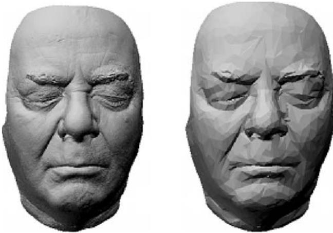
**Fig. 19.** Example of a dense model (*left*) and its shape-preserving simplified model (*right*, 2000 triangles)
