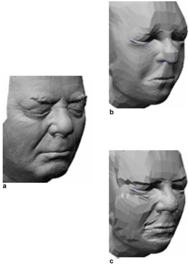
Fig. 6a–c. Comparison of results before and after mesh refinement. **a** Dense model; **b** Working model before refinement; **c** Working model after refinement
