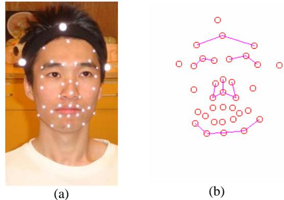
Figure 4 : Facial motion capture using a *VICON*<sup>TM</sup> system. (a) Sparse markers are attached to the subject's face; (b) 3D virtual markers reconstructed by the *VICON*<sup>TM</sup> system.
