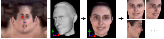
Figure 3: Detected feature points in the texture image are mapped to the 3D mesh model, which is aligned to the frontal view and then rendered with various view directions.
