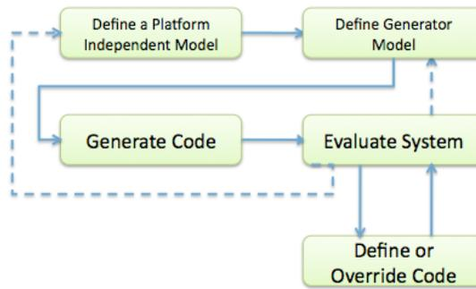
**Figure 12: Software Development Workflow using EMF**
