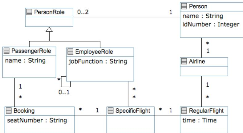
**Figure 2: Airline Reservation System UML Class Diagram [2]**
