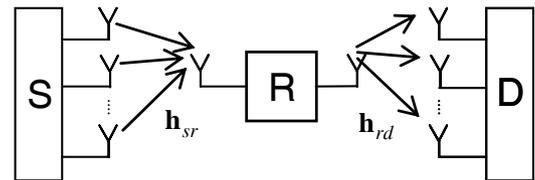
Fig. 1. Relay channel with a single relay node (R) (single-antenna) and multiple-antenna source (S) and destination (D).
