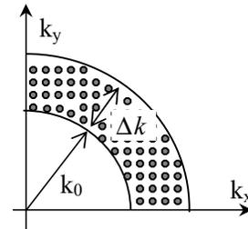
Fig. 4. 2-D illustration of wavenumber space filling.
