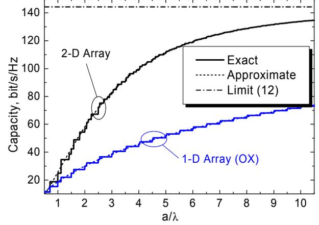
Fig. 3. MIMO capacity in a rectangular waveguide for  $a=b$  and SNR=20 dB.
