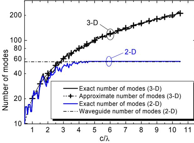
Fig. 5. Number of orthogonal modes in a rectangular cavity for  $a=4\lambda$ ,  $b=2\lambda$  and  $\Delta f/f_0=0.01$ .
