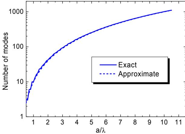
Fig. 7. Number of modes in a circular waveguide.
