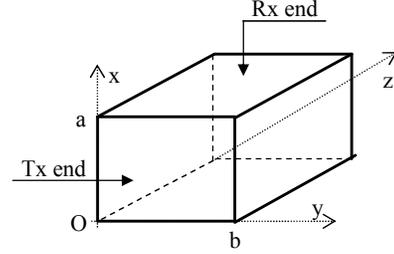
Fig. 1 Rectangular waveguide geometry.
