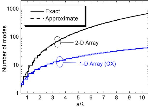
Fig. 2. Number of modes in a rectangular waveguide for  $a=b$ .
