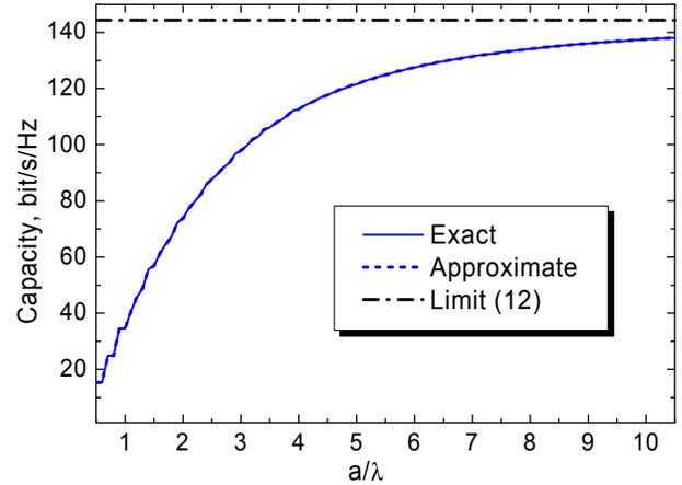
Fig. 8. MIMO capacity in a circular waveguide for SNR=20 dB.
