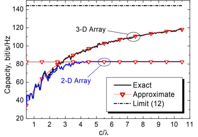
Fig. 6. Capacity in a rectangular cavity for  $a=4\lambda$ ,  $b=2\lambda$  and  $\Delta f/f_0=0.01$ .
