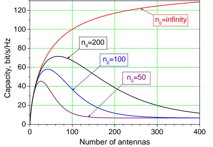
Fig. 2. BLAST channel capacity versus number of antennas,  $\rho=20$  dB.
