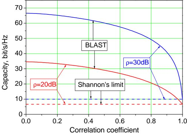
Fig. 1. BLAST channel capacity versus correlation coefficient,  $n=10$ .
