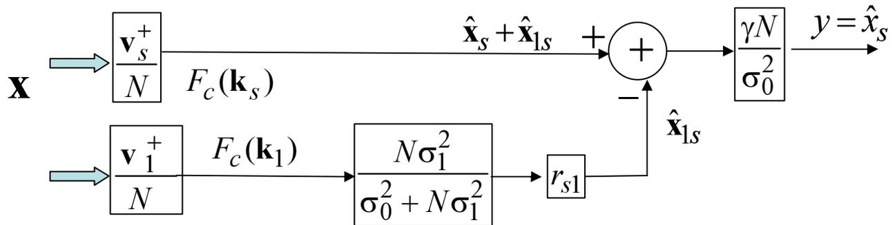
Note that the upper part forms a beam at  $\mathbf{k}_s$ , the lower part forms a beam at  $\mathbf{k}_1$ , and finally, the interferer contribution is subtracted out. This is a sidelobe cancellation.
