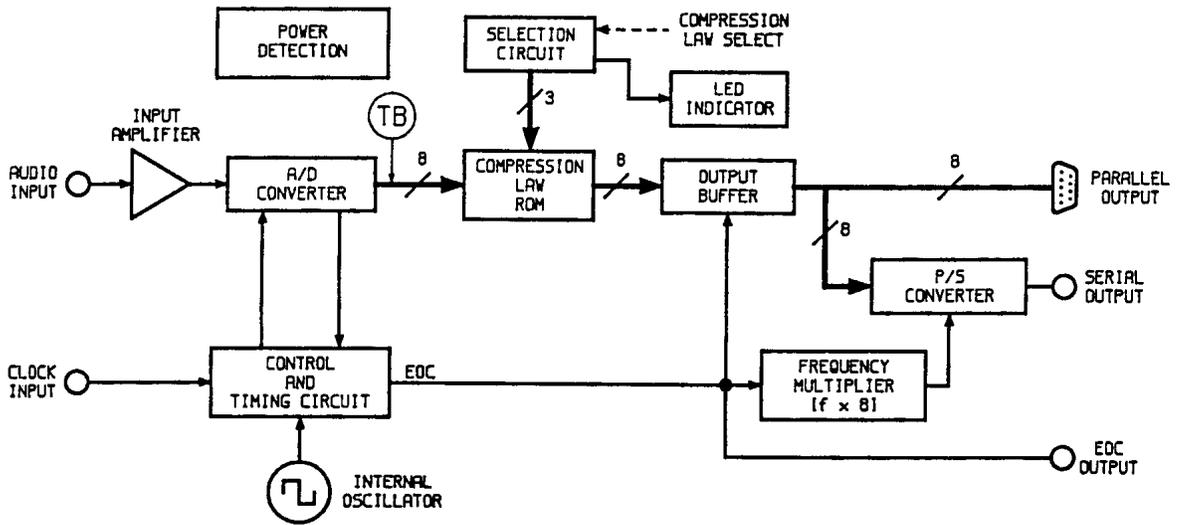
Figure 3. Location of the Test Bus.
