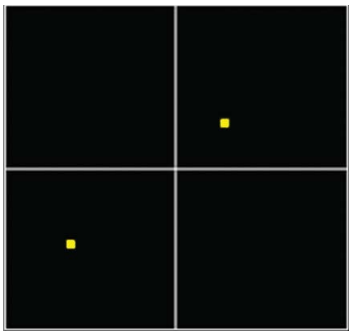
Figure 26. Waveform where the sample rate yields two data points per period
