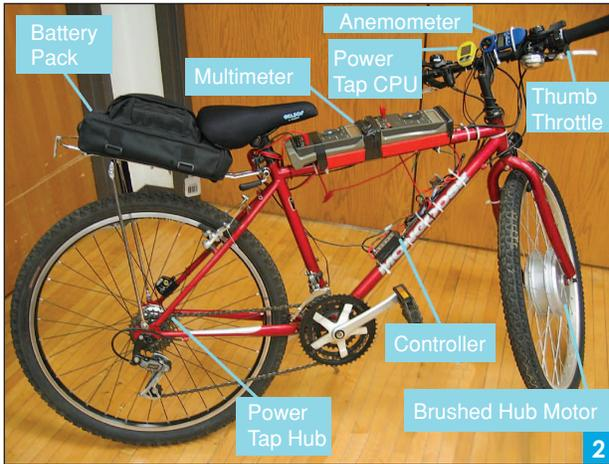
**Electric bicycle test set-up used for the experimental investigation.**
