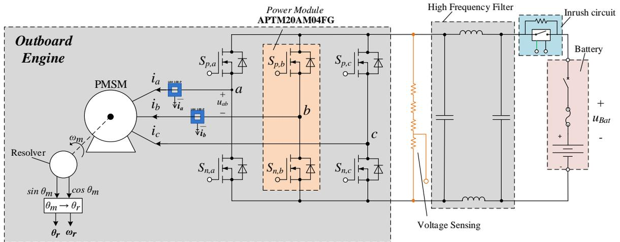
Fig. 4: Propulsion system power structure.
