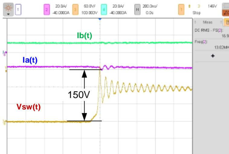
Fig. 12: MOSFET overvoltage – Dead time  $2\mu\text{s}$ .
