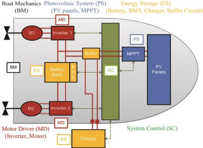
Fig. 1: Electric diagram of the all-electric boat.
