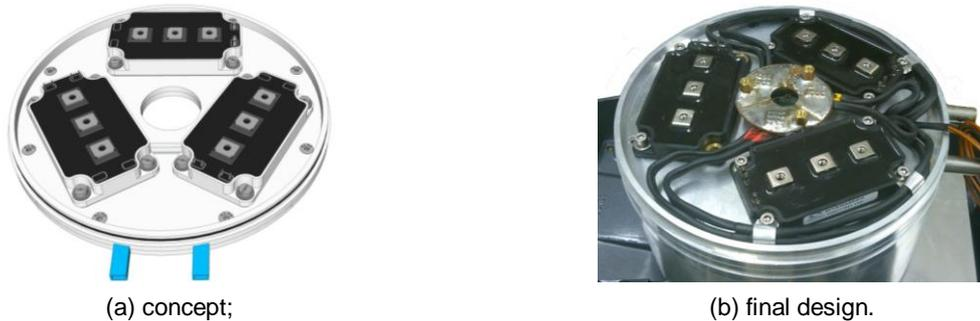
Fig. 9: Proposed water cooled heat sink and power inverter modules.
