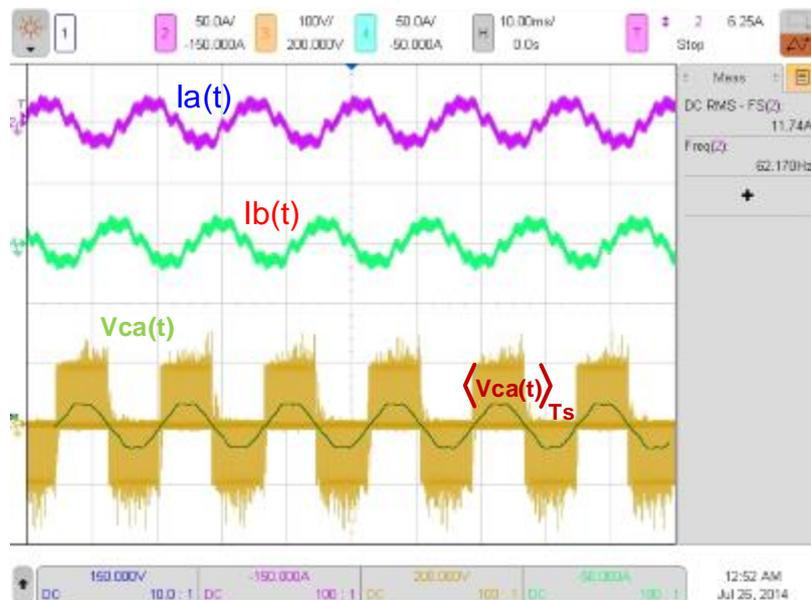
Fig. 10: PMSM waveforms: input voltage and currents.
