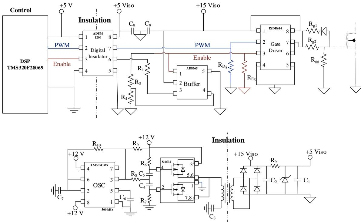
Fig. 6: Circuit used on the MOSFET gate drivers.
