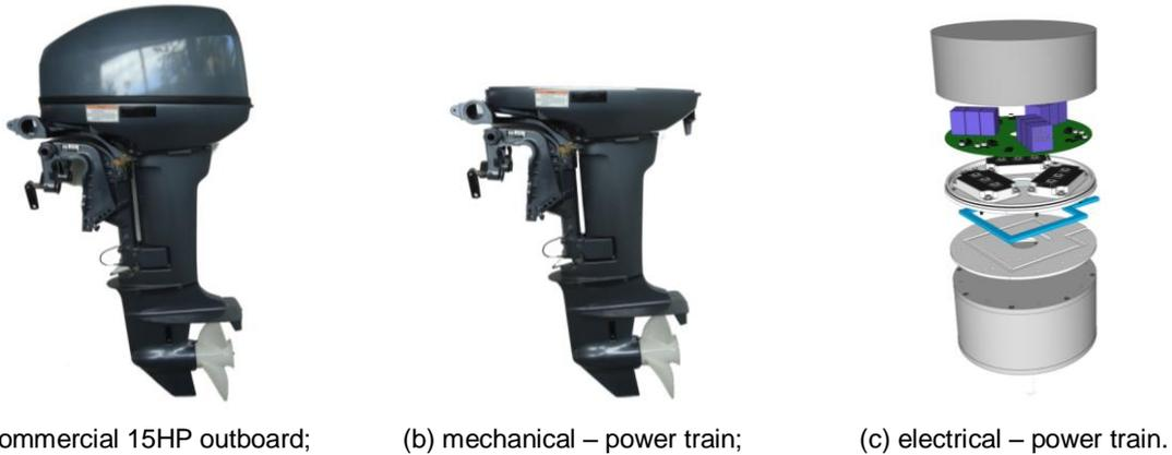
Fig. 2: Electric propulsion system.
