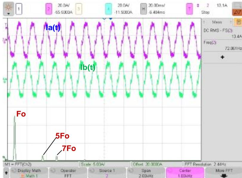
Fig. 11: Phase current harmonics.
