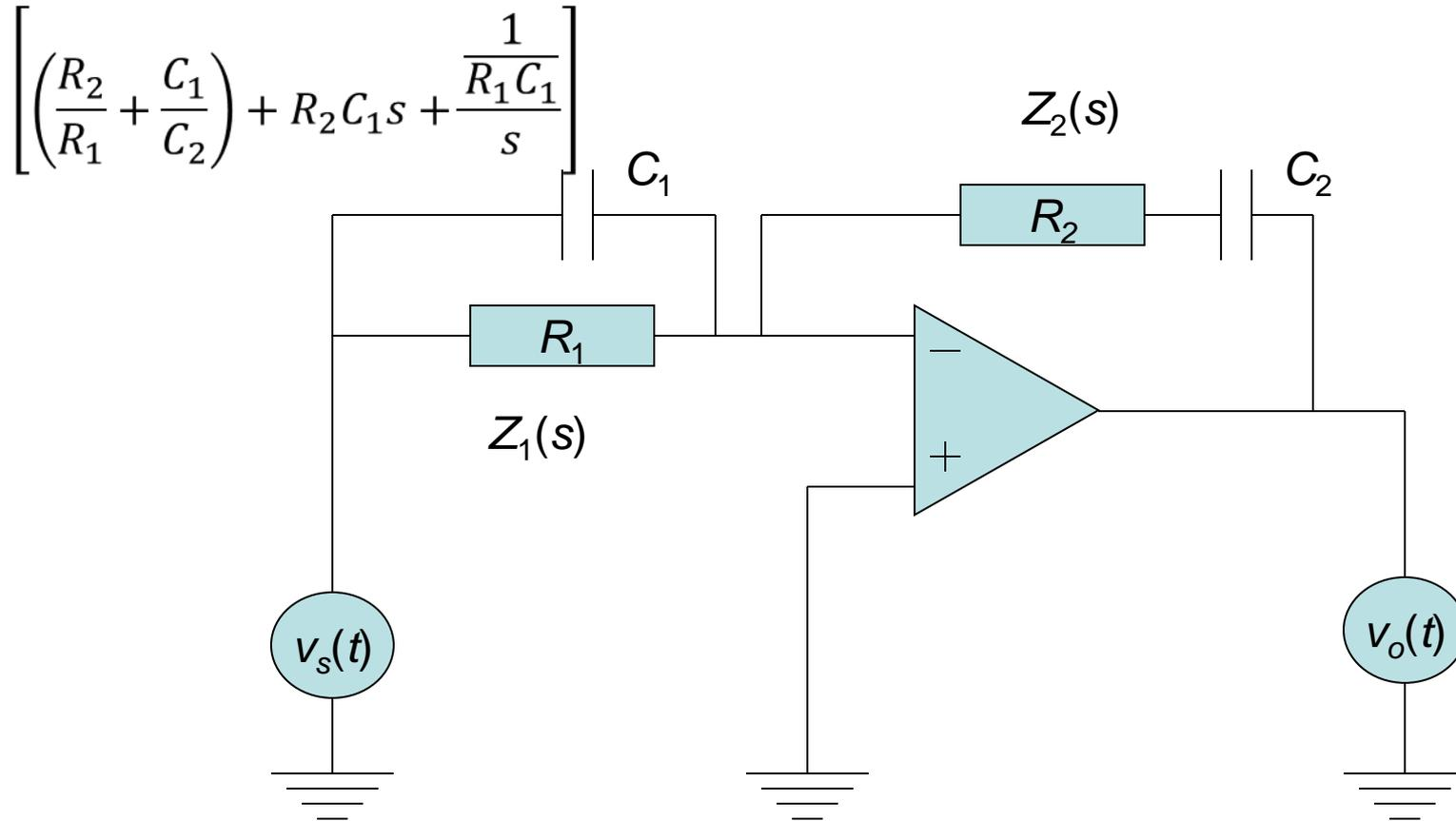
$$G(s) = \frac{V_o(s)}{V_s(s)} = - \frac{(R_1 C_1 s + 1)(R_2 C_2 s + 1)}{R_1 C_2 s} = \frac{R_2 C_1 s^2 + \frac{R_1 C_1 + R_2 C_2}{R_1 C_2} s + \frac{1}{R_1 C_2}}{s}$$
