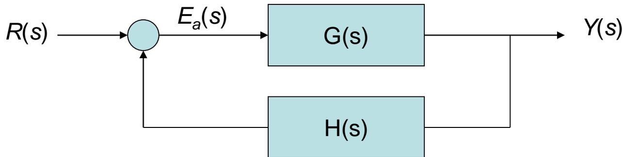
$$E(s) = R(s) - Y(s) = R(s) - \frac{G(s)}{1 + GH(s)} R(s) = \frac{1}{1 + G(s)} R(s) \text{ When } H(s) = 1$$
