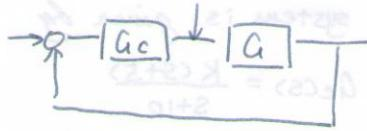
using the ITAE performance method for a step input determine the required  $G_c(s)$ . Assume  $\omega_n = 20$ . Determine the step response with and without a prefilter  $G_p(s)$ .
