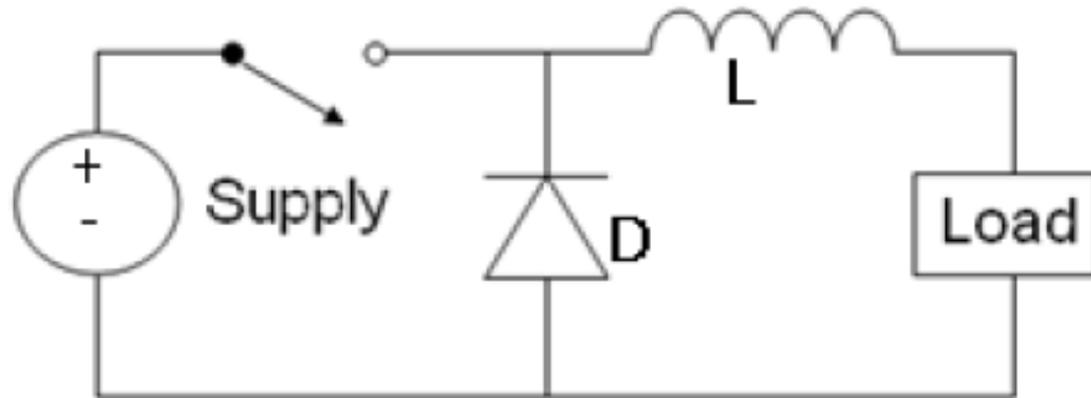
When the switch is closed, the voltage across the inductor is  $V_L = V_i - V_o$ . The current through inductor linearly rises. The diode does not allow current to flow through it, since it is reverse-biased by voltage  $V$ .
