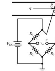
**Hot-wire anemometer:** A heated wire is cooled by the gas flow. The resistance of the wire changes with temperature.
