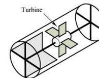
**Turbine flowmeter:** Fluid flow induces rotation of the turbine; measurement of turbine velocity provides an indication of flow rate.
