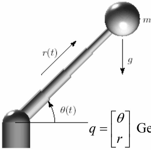
$q = \begin{bmatrix} \theta \\ r \end{bmatrix}$  Generalized coordinates ( $\theta$  angular position;  $r$  radial length; both vary)
