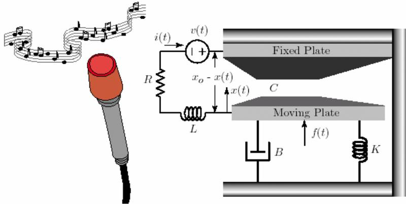
This system has two degrees of freedom (electrical and mechanical : charge  $q$  and displacement  $x$  from equilibrium)
