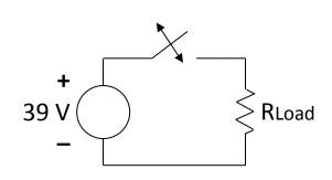
Switch state, Load voltage Closed, 39 V Open, 0 V
