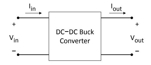
Lossless objective:  $P_{in} = P_{out}$ , which means that  $V_{in}I_{in} = V_{out}I_{out}$
