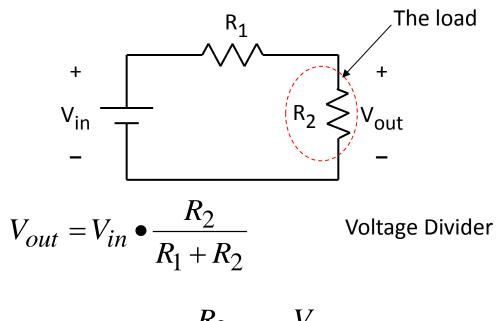
$$\eta = \frac{R_2}{R_1 + R_2} = \frac{V_{out}}{V_{in}}$$
