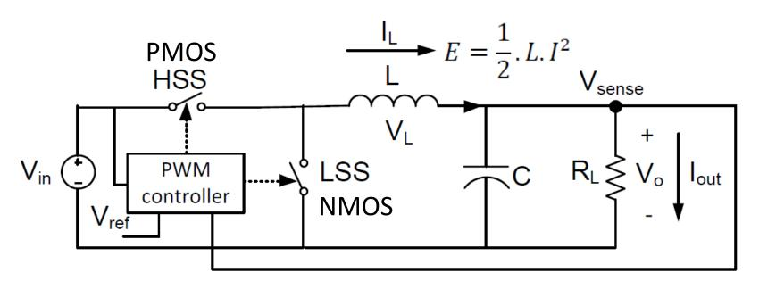
$$D = \frac{t_{on}}{T} = \frac{t_{on}}{t_{on} + t_{off}} = f_{sw}.t_{on}$$
