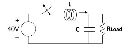
Try adding an L to prevent the huge current spike. But now, if the L has current when the switch attempts to open, the inductor's current momentum and resulting *Ldi/dt* burns out the switch.
