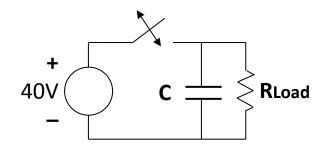
Try adding a large C in parallel with the load to control ripple. But if the C has 13Vdc, then when the switch closes, the source current spikes to a huge value and burns out the switch.
