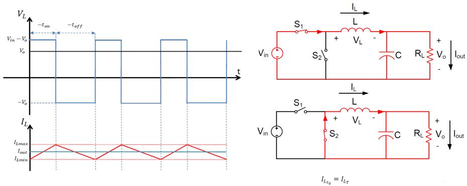
$$\Delta I_{L_{ON}} = \int_0^{t_{ON}} \frac{V_L}{L} dt = \frac{(V_{in} - V_o)}{L} t_{ON}$$
