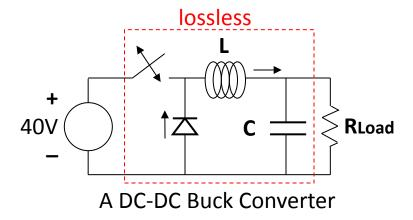
By adding a "free wheeling" diode, the switch can open and the inductor current can continue to flow. With high-frequency switching, the load voltage ripple can be reduced to a small value.
