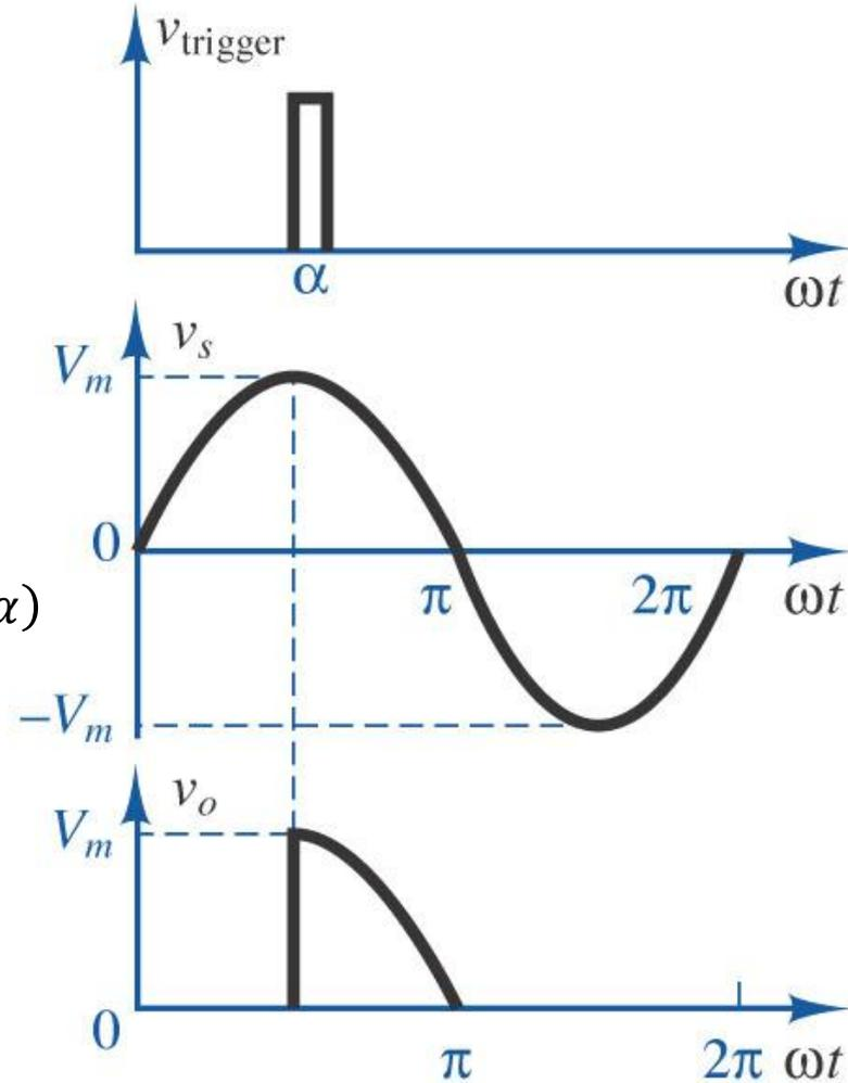
$$V_{dc} = \frac{1}{2\pi} \int_{\alpha}^{\pi} V_p \sin \omega t d\omega t = \frac{V_p}{2\pi} (1 + \cos \alpha)$$
