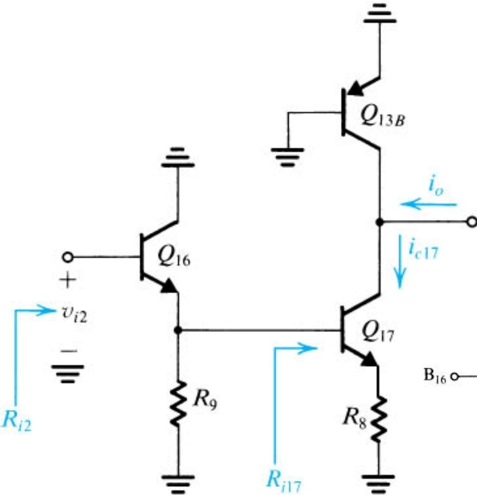
$$R_{o2} = (R_{o13B} \parallel R_{o17}) = 81 \text{ k}\Omega$$
