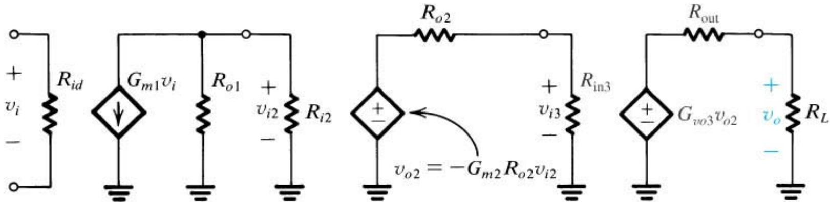
$$\frac{v_o}{v_i} = \frac{v_{i2}}{v_i} \frac{v_{o2}}{v_{i2}} \frac{v_o}{v_{o2}}$$
