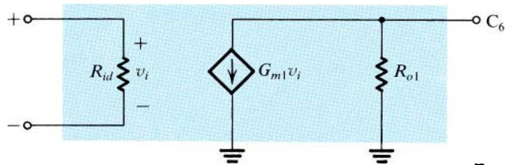
Example: Determine the small-signal differential voltage gain of the 741 op-amp input stage. Assume transistor gain of  $\beta = 200$  and Early voltages of  $V_A = 50$  V.
