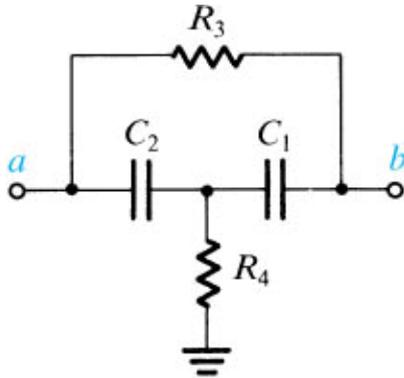
$$t(s) = \frac{s^2 + s\left(\frac{1}{C_1} + \frac{1}{C_2}\right)\frac{1}{R_3} + \frac{1}{C_1 C_2 R_3 R_4}}{s^2 + s\left(\frac{1}{C_1 R_3} + \frac{1}{C_2 R_3} + \frac{1}{C_1 R_4}\right) + \frac{1}{C_1 C_2 R_3 R_4}}$$
