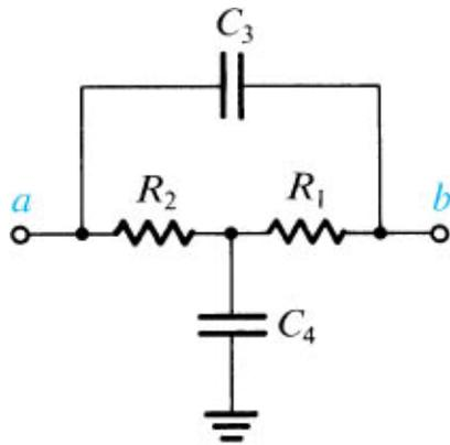
$$t(s) = \frac{s^2 + s\left(\frac{1}{R_1} + \frac{1}{R_2}\right)\frac{1}{C_4} + \frac{1}{C_3 C_4 R_1 R_2}}{s^2 + s\left(\frac{1}{C_4 R_1} + \frac{1}{C_4 R_2} + \frac{1}{C_3 R_2}\right) + \frac{1}{C_3 C_4 R_1 R_2}}$$
