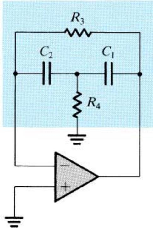
$$s^2 + s \frac{\omega_0}{Q} + \omega_0^2 = s^2 + s \left( \frac{1}{C_1} + \frac{1}{C_2} \right) \frac{1}{R_3} + \frac{1}{C_1 C_2 R_3 R_4}$$
