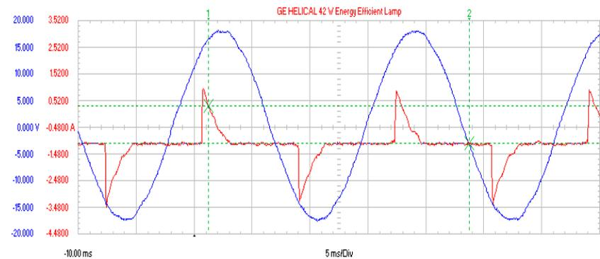
The waveforms show the voltage in blue and the pulses of current from an energy efficient GE HELICAL 42 W lamp
