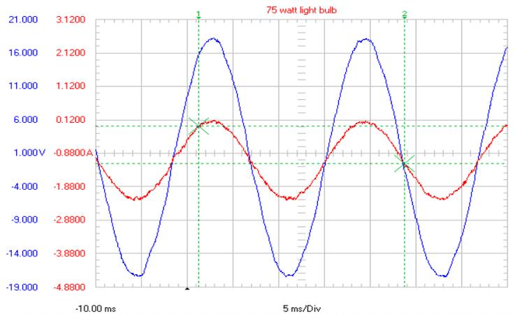
Waveforms of a 75 watt incandescent light bulb
