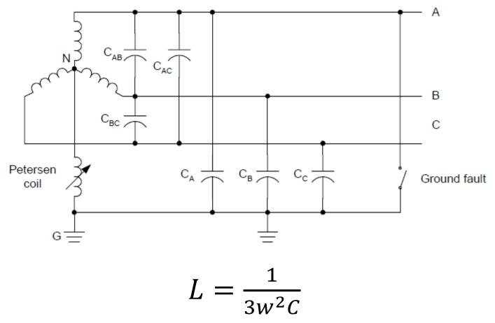
This condition states that the inductance must be tuned to the capacitance if the Peterson coil is to fulfill its function.
