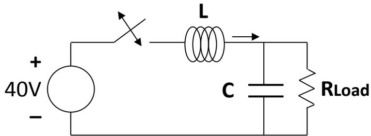
Try adding an L to prevent the huge current spike. But now, if the L has current when the switch attempts to open, the inductor's current momentum and resulting  $Ldi/dt$  **burns out the switch**.
