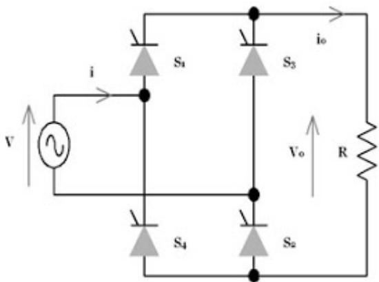
$$V_{dc} = \frac{2}{2\pi} \int_{\alpha}^{\pi+\alpha} V_p \sin \omega t d\omega t = \frac{2V_p}{\pi} (\cos \alpha)$$
