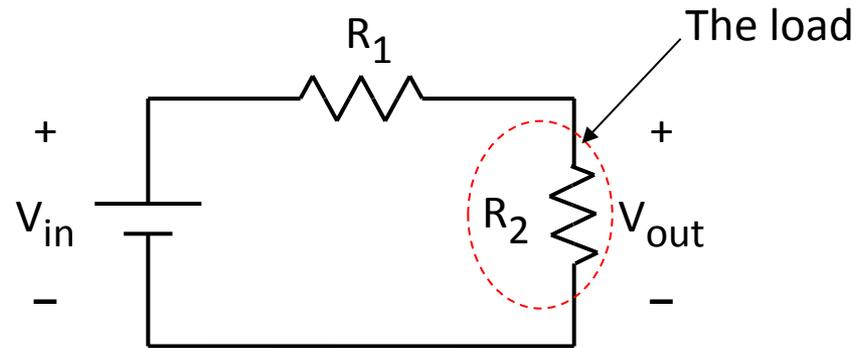
$$V_{out} = V_{in} \cdot \frac{R_2}{R_1 + R_2} \quad \text{Voltage Divider}$$
