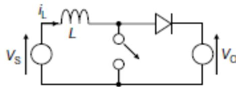
boost converter operating into a voltage source
