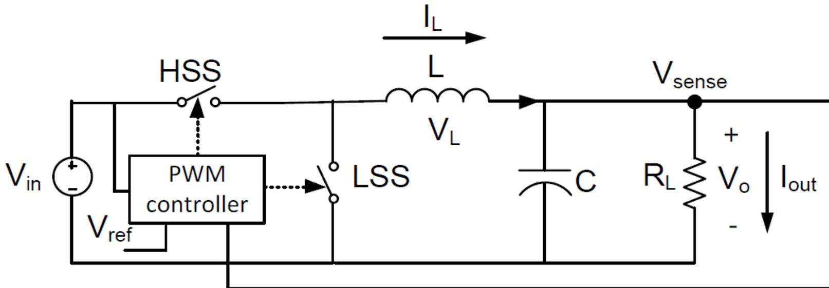
$$D = \frac{t_{on}}{T} = \frac{t_{on}}{t_{on} + t_{off}} = f_{sw} \cdot t_{on}$$
