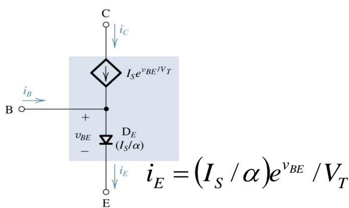
Voltage - controlled Current Source (a)
