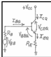
$$V_{BB} = V_{CC} \frac{R_2}{R_1 + R_2} = 12 \frac{22}{22 + 82} = 2.538 \text{ V}$$
