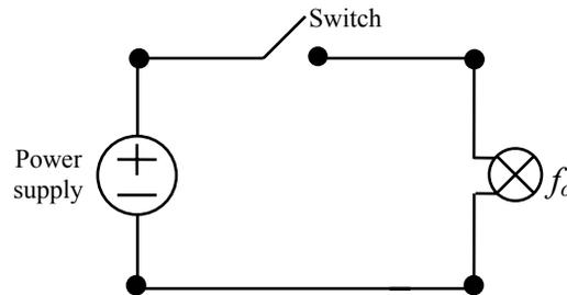
**Figure 2** Electric circuit with a switch.
