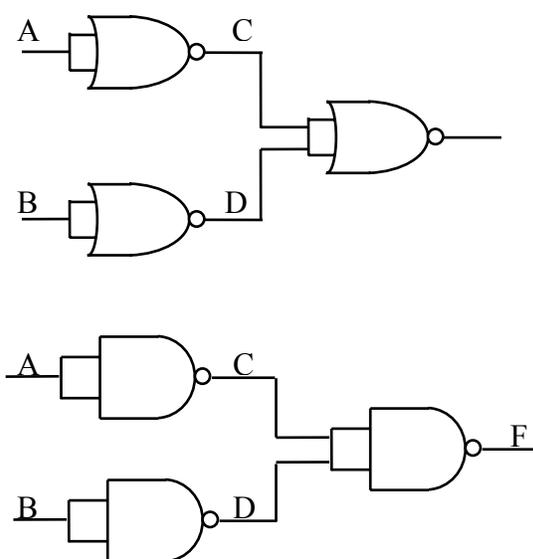
**Figure 8** Three NOR and three NAND circuits.
