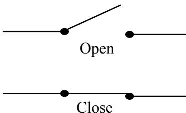
**Figure 1** Two conditions for a simple switch.
