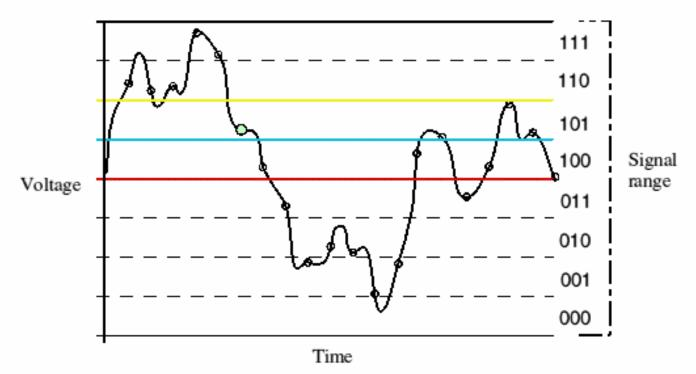
Turning analog waves into digital signals.
