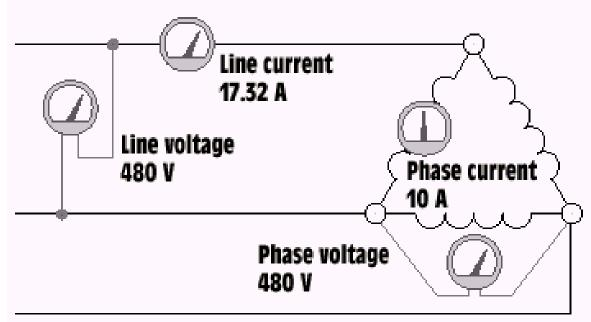
Example 1: A Y-connected three phase generator (line voltage of 480 V) supplies power to a delta-connected resistive load (8  $\Omega$  each). Find E<sub>L(load)</sub>, E<sub>P(load)</sub>, and I<sub>P(load)</sub>, I<sub>L(load)</sub>, I<sub>L(gen)</sub>, E<sub>P(gen)</sub>, and the true power.
