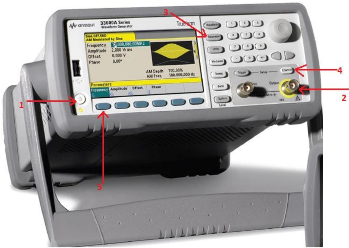
**Figure 3:** Digital function generator.
