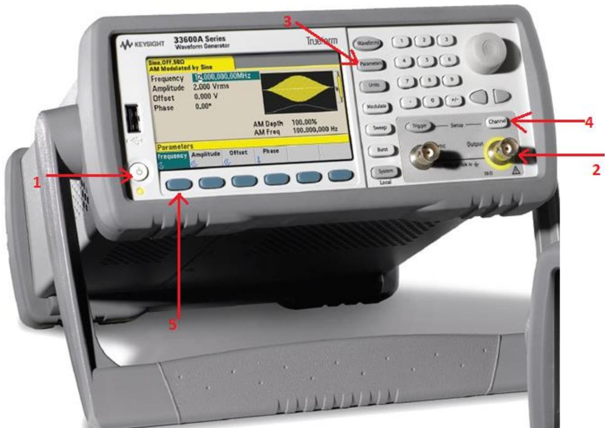
**Figure 3:** Digital function generator.
