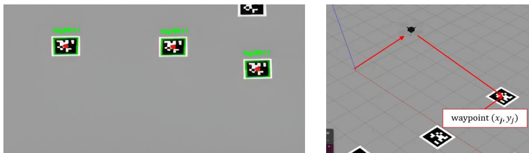
Fig. 1: Locations of interest and waypoints determination from a UAV embedded vision sensor looking downward.
