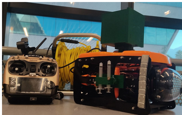
Fig. 6: Mounting the device as an appendage to a remotely operated underwater vehicle.
