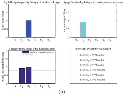
Figure 4: a) Assigning agent  $R_3$  to a task of type 2 on water-covered area, and b) specialty fitting scores of the available robots and minimum fitting threshold w.r.t. the current task.
