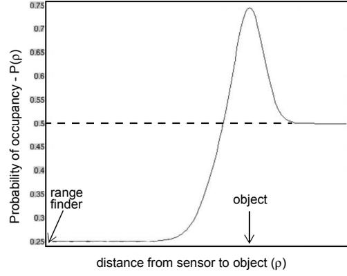
Fig. 1. Range sensor model with Gaussian uncertainty.
