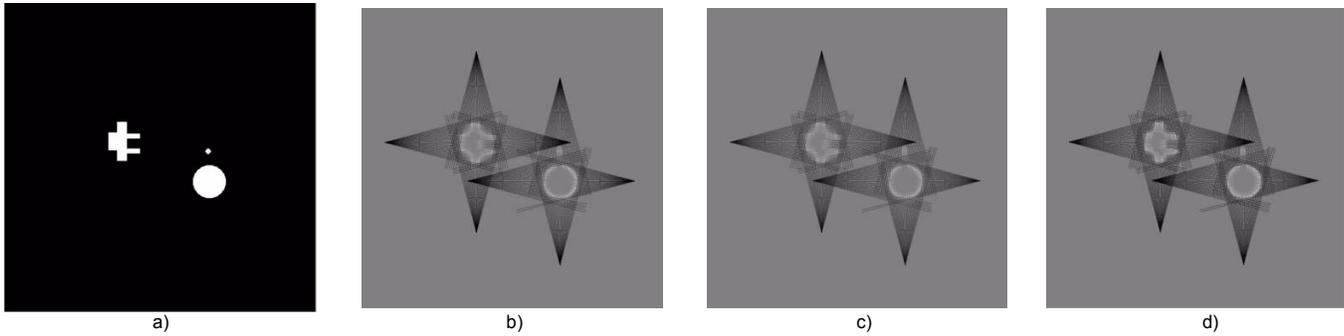
Fig. 9. 2D certainty maps resulting for the merge of range measurements from 8 viewpoints on a) a predefined environment, using b) the Bayesian theorem, c) the Dempster-Shafer theory of evidence, and d) the fuzzy logic inference engine.
