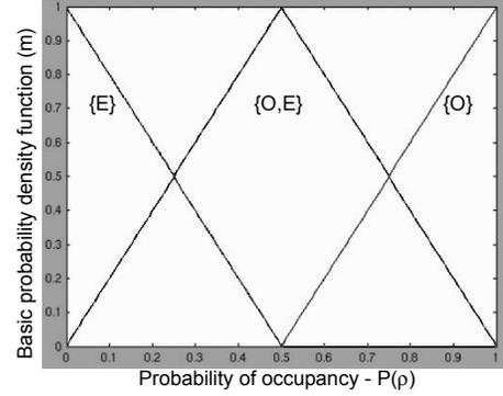
Fig. 3. Conversion between the Gaussian sensor uncertainty model and the basic probability density function of Dempster-Shafer.
