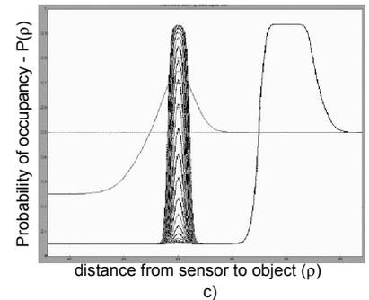
Fig. 5. Progressive model refinement with Dempster-Shafer theory of evidence.
