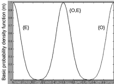
Fig. 4. Conversion from the Dempster-Shafer mapping to a probabilistic occupancy representation.
