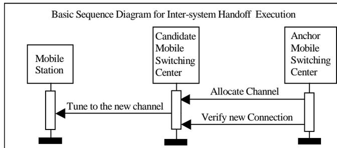
Figure 13. A scenario for the *Inter-System Handoff Execution*
