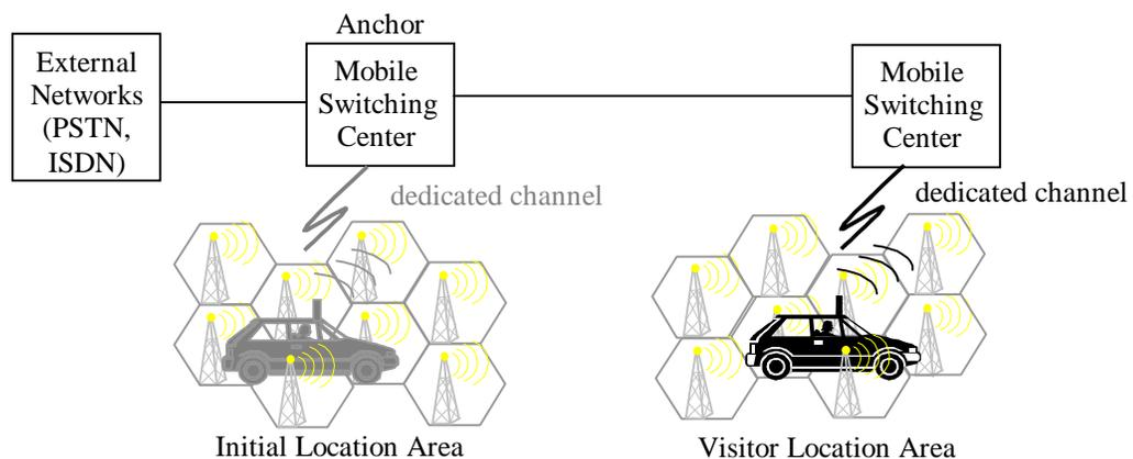
Figure 12. ANSI-41 Successful Handoff-Forward with *Anchor entity* [8]
