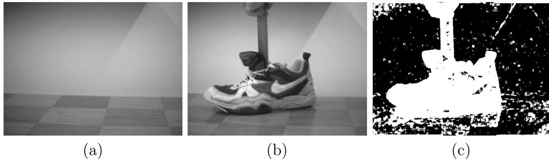
Figure 6.3: (a) Background for the right camera of the *Running Shoe* sequence (b) Sample of the *Running Shoe* sequence (c) Extracted silhouette with three distinctive features: rounding effect by the use of correlation windows, false negative “holes” and false positive “snow”
