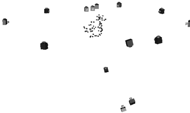
Figure 7: Positions of the left camera in the Duck sequence, as computed by PhotoModeler.
