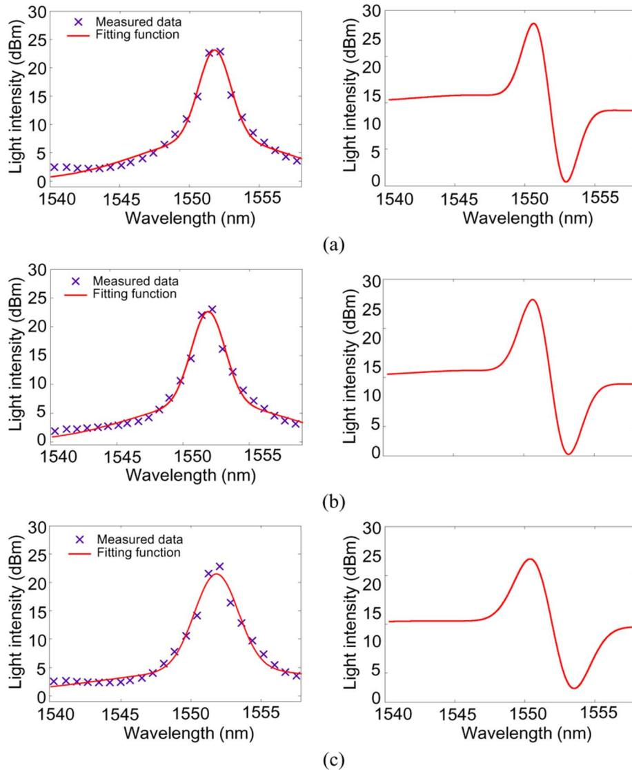
Fig. 6. Curve fitting functions (left) and the first-order derivatives (right) for three different strains applied to the LPG. (a) LPG without strain. (b) LPG with Strain 1. (c) LPG with Strain 2.
