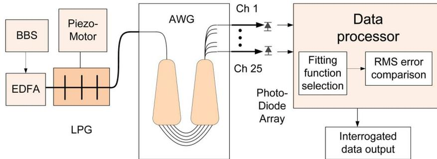
Fig. 3. An LPG sensor interrogation system using an AWG.
