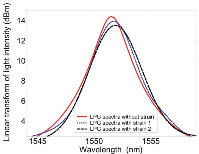
Fig. 5. LPG spectra with different strains.
