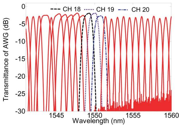
Fig. 4. The transmission spectrum of the AWG. The dashed line, dotted line and dash-dot line show the spectra for Channels 18, 19, and 20, respectively.
