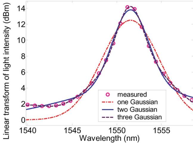
Fig. 2. Curve fitting of the spectra of the resonant dip of LPG2 using a linear combination of one, two, and three Gaussian functions.
