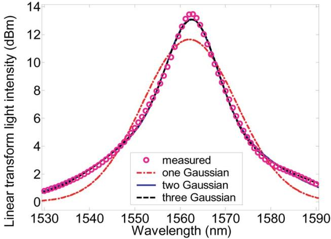
Fig. 1. Curve fitting of the spectra of the resonant dip of LPG1 using a linear combination of one, two, and three Gaussian functions.
