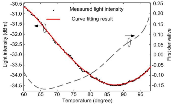
Fig. 4. Detected light intensity, curve fitting, and the first-order derivative versus the chip temperature.
