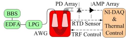
Fig. 2. Experimental setup for LPG interrogation based on a thermally tunable AWG.
