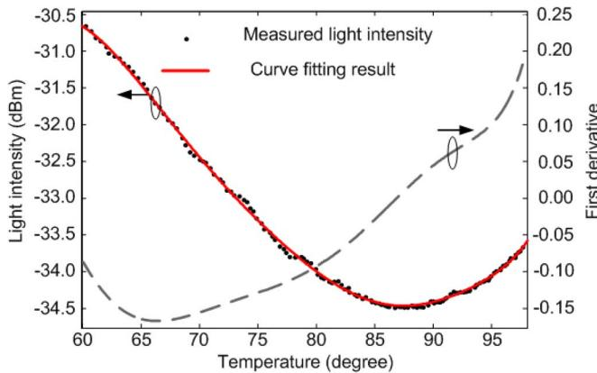
Fig. 4. Detected light intensity, curve fitting, and the first-order derivative versus the chip temperature.
