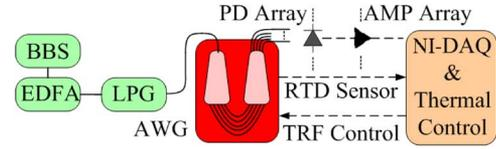
Fig. 2. Experimental setup for LPG interrogation based on a thermally tunable AWG.
