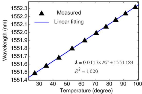
Fig. 1. Experimental result of the temperature dependence of a selected AWG channel.
