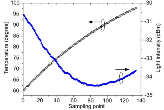
Fig. 3. Experimental results for LPG interrogation measured from the DAQ card.
