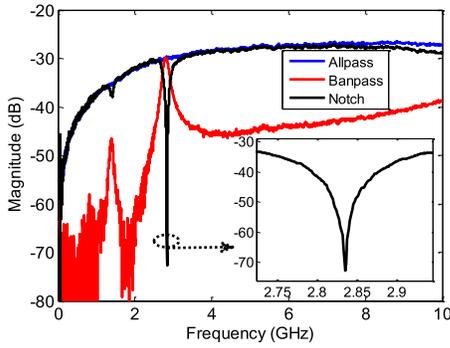
Fig. 3. Frequency responses of the allpass filter, the bandpass filter, and the corresponding notch filter.
