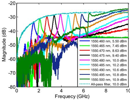
Fig. 4. Frequency response of the allpass filter and the bandpass filter with the power of the bandpass filter adjusted to match the power of the allpass filter.
