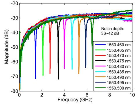
Fig. 5. Frequency response of the proposed notch filter with the allpass power kept constant and the power of the bandpass filter adjusted to match the power of the allpass filter.
