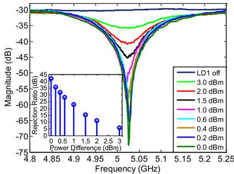
Fig. 9. Frequency response to show the tuning of the notch depth. Inset: relationship between the notch depth and the power difference.
