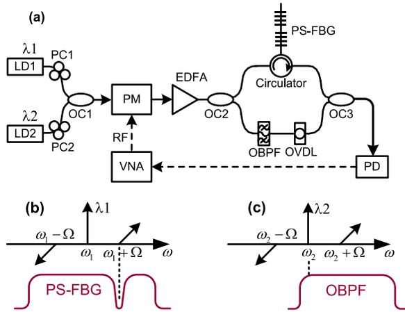
Fig. 1. (a) Schematic of the proposed single-notch MPF. (b) The spectral relationship between the phase-modulated signal and the PS-FBG. (c) The spectral relationship between the phase-modulated signal and the OBPF.
