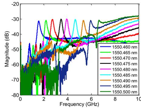
Fig. 6. Frequency response of the bandpass filter with the power kept constant.
