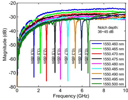
Fig. 8. Frequency response of the proposed notch filter with the bandpass power kept constant and the power of the allpass filter adjusted to match the power of the bandpass filter.
