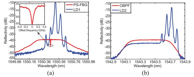
Fig. 2. The spectra of (a) the phase-modulated signal at the output of the PS-FBG, and (b) the phase-modulated signal at the output of the OBPF.
