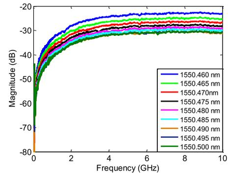
Fig. 7. Frequency response of the allpass filter with the power adjusted to match the power of the bandpass filter.
