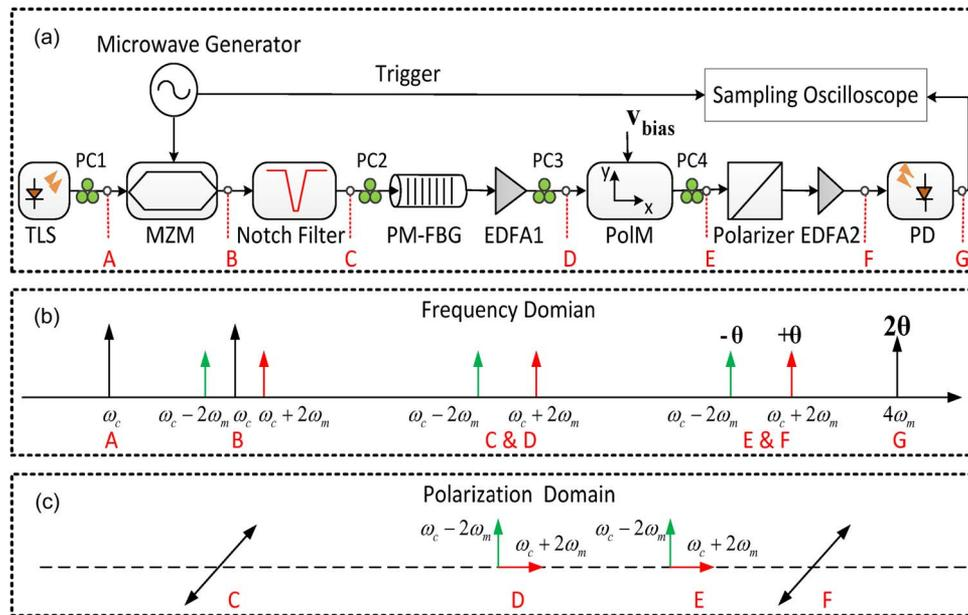
Fig. 1. (a) Schematic of the proposed system for mm-wave signal generation with tunable phase shift. (b) Illustration of the operation principle in the frequency domain, and (c) evolution of the polarization states.
