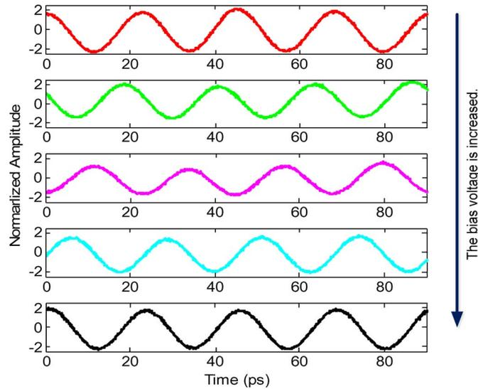
Fig. 4. Temporal waveforms of the generated 44-GHz mm-wave signal at different bias voltages measured using a sampling oscilloscope. When the voltage is tuned, the 44-GHz waveform is laterally shifted corresponding a shift in phase.
