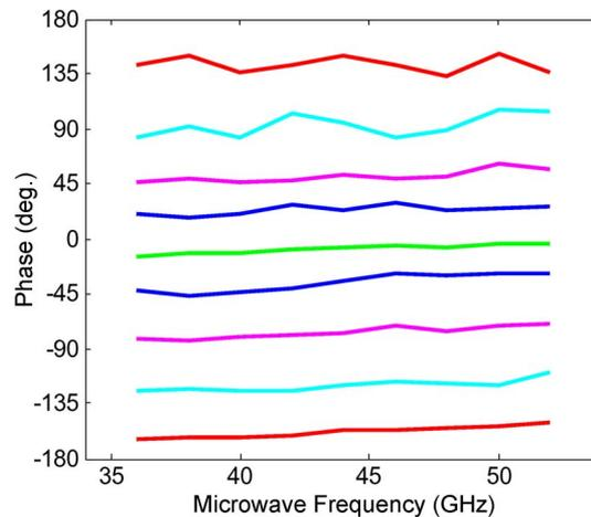
Fig. 5. Measured phase shifts at different bias voltages over a microwave frequency band from 36 to 52 GHz. The phase shifts are independent of the microwave frequency.
