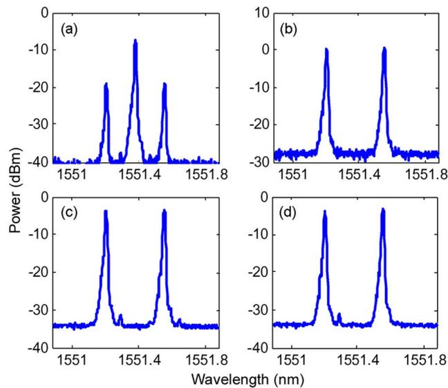
Fig. 3. Measured spectra using an optical spectrum analyzer at the output of the (a) MZM; (b) PM-FBG; (c) PolM; and (d) Polarizer.
