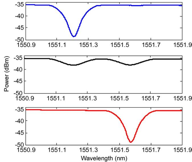
Fig. 2. Transmission spectra of the PM-FBG measured using a broadband light source with its polarization direction oriented at an angle of  $0^\circ$ ,  $45^\circ$ , and  $90^\circ$  to the fast axis of the PM-FBG.
