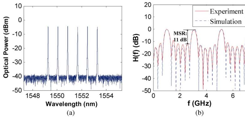
Fig. 5. Frequency response of a six-tap filter with coefficients of  $[1 -1 1 -1 1 -1]$ . (a) Optical spectrum of the six light waves sent to the PoIM with a frequency spacing of 100 GHz (0.8 nm), and (b) the corresponding frequency response of the six-tap microwave photonic filter.
