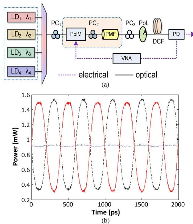
Fig. 3. (a) Experimental setup of the proposed microwave photonic filter. (b) Generation of two complementary microwave optical signals. LD: laser diode, PC: polarization controller, PoIM: polarization modulator, PMF: polarization-maintaining fiber, Pol.: polarizer, DCF: dispersion-compensating fiber, VNA: vector network analyzer, PD: photodetector.
