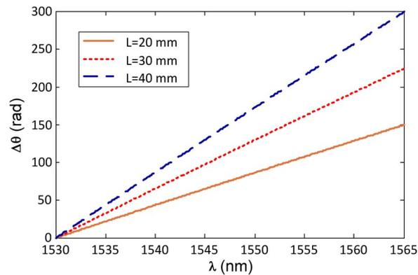
Fig. 2. Phase difference versus wavelength relative to a reference wavelength of 1530 nm for a  $\text{LiNbO}_3$  crystal in the phase modulator with a length of 20, 30, and 40 mm.
