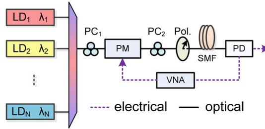
Fig. 1. Schematic of the proposed microwave photonic filter. LD: laser diode, PC: polarization controller, PM: phase modulator, Pol.: polarizer, VNA: vector network analyzer, PD: photodetector.
