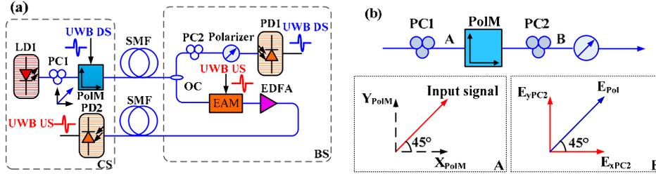
Fig. 1. (a) A bidirectional UWBof system with wavelength reuse for upstream transmission. (b) Equivalent MZM using a PolM, a PC and a polarizer.
