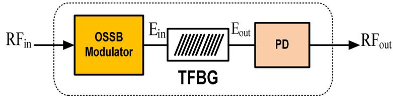
Fig. 3. Schematic block diagram of the proposed phase shifter. OSSB: optical signal-sideband, PD: photodetector.
