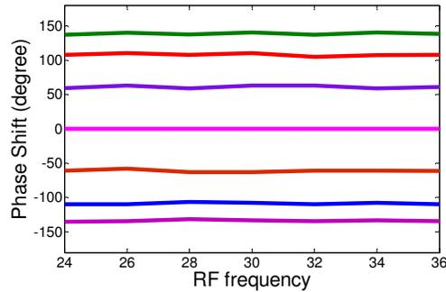
Fig. 6. Measured phase shifts at different pumping power levels. The phase shifts are independent of the microwave frequency.
