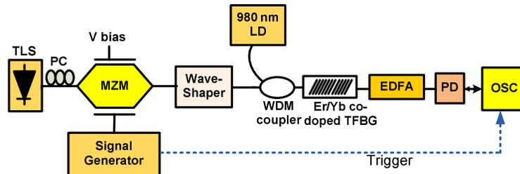
Fig. 4. Experimental setup. TLS: tunable laser source, PC: polarization controller, MZM: Mach-Zehnder modulator, LD: laser diode, WDM: 980/1550 nm wavelength division multiplexer, EDFA: erbium-doped fiber amplifier, PD: photo-detector, OSC: oscilloscope.
