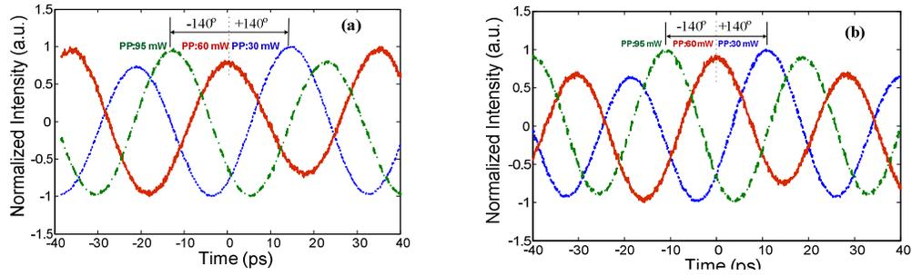
Fig. 5. The detected signals at pump power levels of 30, 60 and 95 mW for the RF frequency of 28 GHz, and (b) 34 GHz. PP: pumping power.
