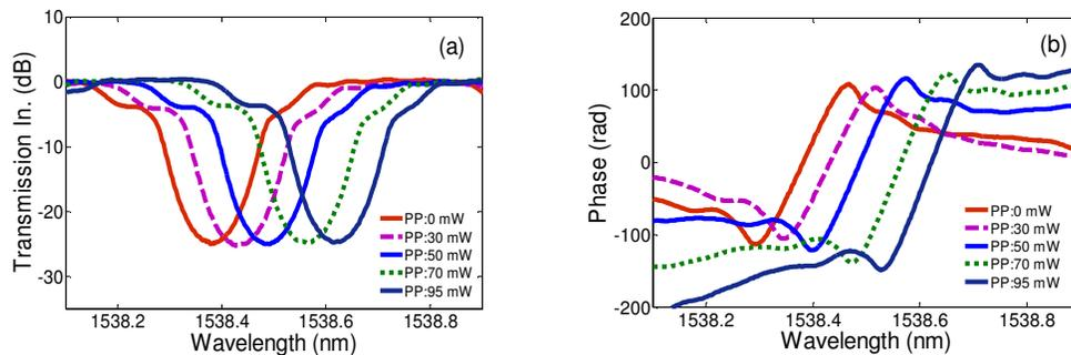
Fig. 2. (a) The magnitude response, and (b) the phase response of one cladding-mode resonance channel of the TFBG. PP: pumping power.
