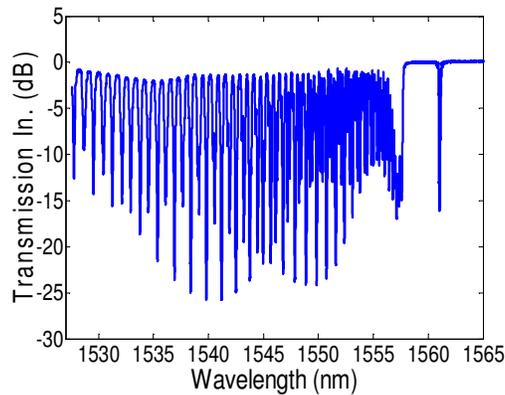
Fig. 1. (a) The transmission spectrum of a TFBG with a tilt angle of  $6^\circ$ , and a Bragg wavelength of 1560 nm.
