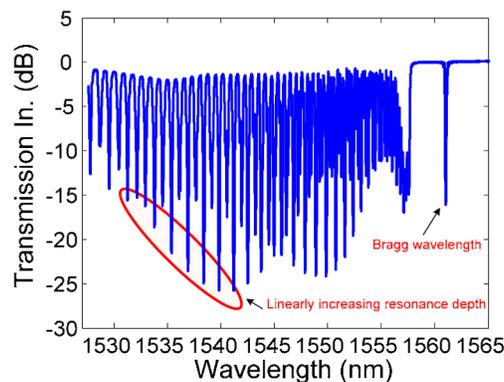
Fig. 1. The transmission spectrum of a TFBG with a tilt angle of  $6^\circ$  and a Bragg wavelength of 1560 nm. The red solid line shows the linear slope of the resonances' depth.
