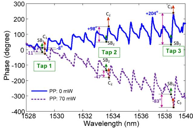
Fig. 2. The phase responses of the TFBG and the placement of the wavelengths of the optical carriers for a three-tap filter at two pumping power levels of 0 and 70 mW.  $C_1$ ,  $C_2$  and  $C_3$  represent the three carriers, and  $SB_1$ ,  $SB_2$  and  $SB_3$  represent the three sidebands.
