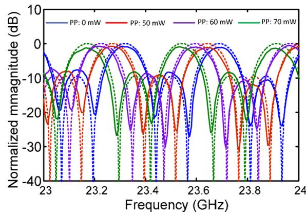
Fig. 4. Frequency response of the three-tap microwave photonic filter with complex coefficients at different pumping power levels (solid lines). The dashed lines show the simulated frequency response corresponding to a basic phase shift of  $+105^\circ$ ,  $+58^\circ$ ,  $+10^\circ$  and  $-36^\circ$ . PP: pumping power.
