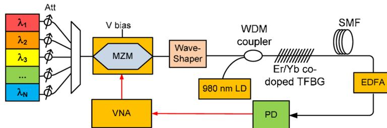
Fig. 3. Experimental setup of the proposed multi-tap microwave photonic filter with complex coefficients. Att: optical attenuator, MZM: Mach-Zehnder modulator, LD: laser diode, WDM: 980/1550 nm wavelength division multiplexer, SMF: single mode fiber, EDFA: erbium-doped fiber amplifier, PD: photodetector, VNA: vector network analyzer.
