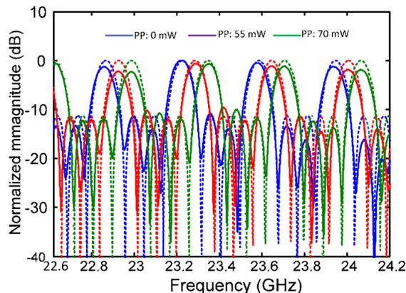
Fig. 5. Frequency response of the four-tap microwave photonic filter with complex coefficients at different pumping power levels (solid lines). The dashed lines show the simulated frequency response corresponding to a basic phase shift of  $-30^\circ$ ,  $+36^\circ$ , and  $+90^\circ$ . PP: pumping power.
