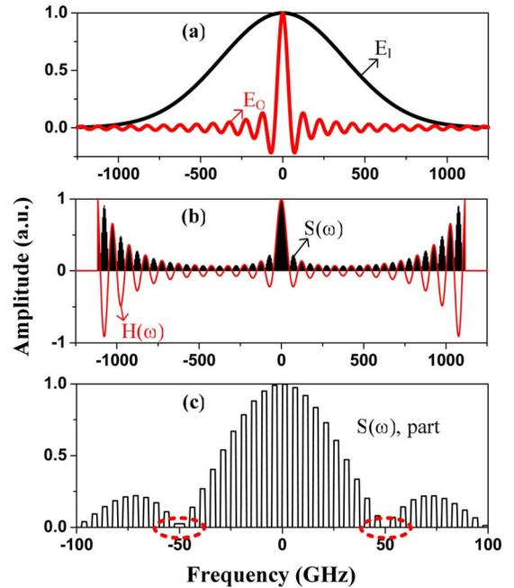
Fig. 2. (Color online) Frequency-domain illustration. (a) Spectra of the input and desired output waveforms. (b) Designed frequency response of a regular  $[H(\omega)]$  and the proposed  $[S(\omega)]$  filters. (c) Zoom-in display of  $S(\omega)$ .
