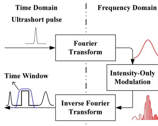
Fig. 1. (Color online) Arbitrary pulse shaping with intensity-only modulation in the frequency domain.
