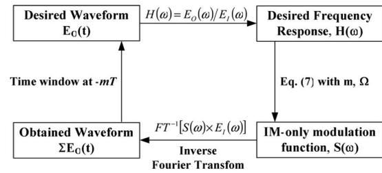
Fig. 4. Flow chart for the design of arbitrary pulse shaping with intensity-only modulation in the frequency domain. IM, intensity modulation.
