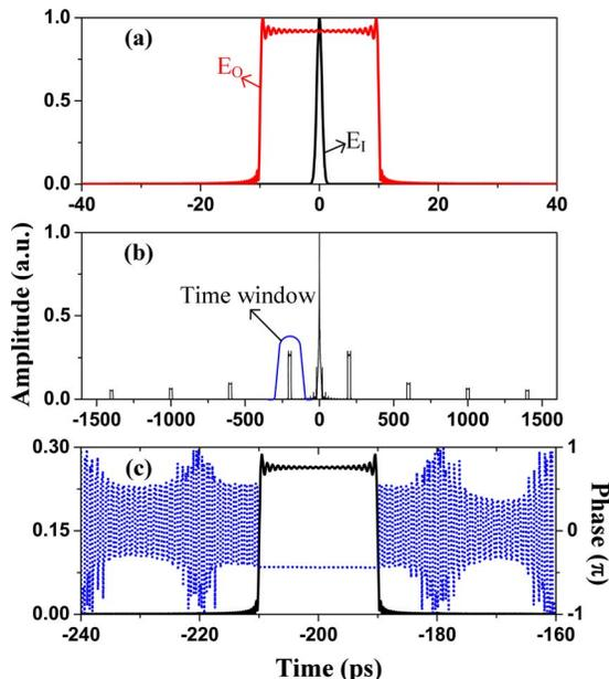
Fig. 3. (Color online) Time-domain illustration. (a) Waveform of the input pulse and the generated pulse by the regular filter  $H(\omega)$ . (b) Generated multiple pulses by the proposed filter  $S(\omega)$ . (c) Generated rectangle waveform selected by a time window and its phase distribution.
