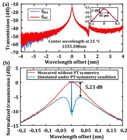
**Fig. 2.** (a) Measured transmission spectra at the corresponding drop ports when the input ports are chosen to be ports A and C at a temperature of 25°C. (b) Equivalent transmission spectrum with a gain contrast enhancement factor  $G$  in the PT-symmetry condition.
