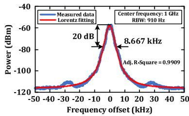
**Fig. 5.** Measured linewidth of the proposed PT-symmetric fiber laser at a wavelength of 1550 nm.
