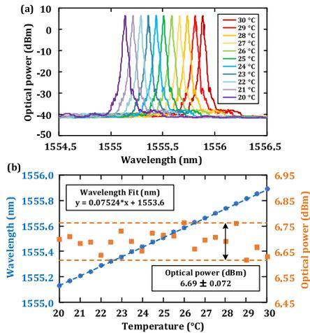
**Fig. 6.** (a) Measured optical spectra by thermally tuning the MDR. (b) Measured center wavelength and the output power of the laser when the MDR is thermally tuned.
