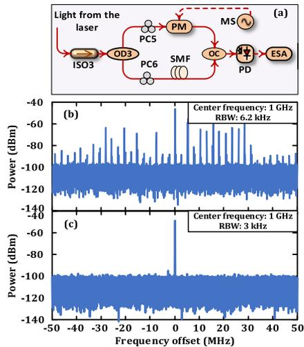
**Fig. 4.** (a) Schematic diagram of a delayed self-heterodyne system. (b) Measured self-heterodyne RF beating spectra at 1555 nm without PT-symmetry and (c) with PT-symmetry. ISO, isolator; OD, optical divider; PC, polarization controller; PM, phase modulator; SMF, single-mode fiber; OC, optical coupler; PD, photodetector; MS, microwave source; ESA, electrical spectrum analyzer.
