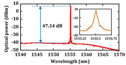
**Fig. 3.** Measured optical spectrum at the output of the PT-symmetric fiber laser.
