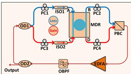
**Fig. 1.** Schematic diagram of the proposed PT symmetric fiber laser. OD, optical divider; PC, polarization controller; MDR, microdisk resonator; PBC, polarization beam combiner; EDFA, erbium-doped fiber amplifier; OBPF, optical bandpass filter.
